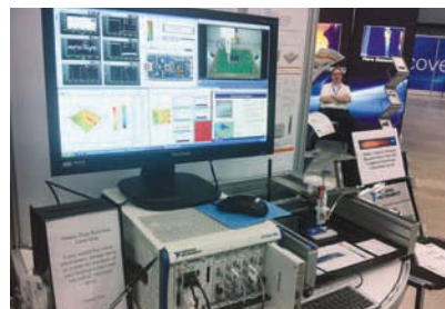
Here’s the full EMI measurement system in operation. On the left is the PXI box with LabView running on top. To the right, the EMI probe measures the EMI directly over an IC.
