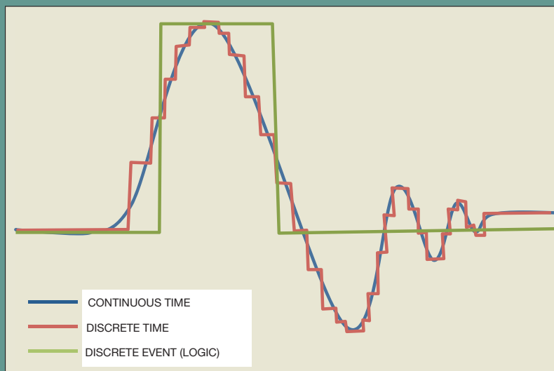
Figure A Various sampling methodologies are compared. Analog simulators break the time axis into small time steps.
